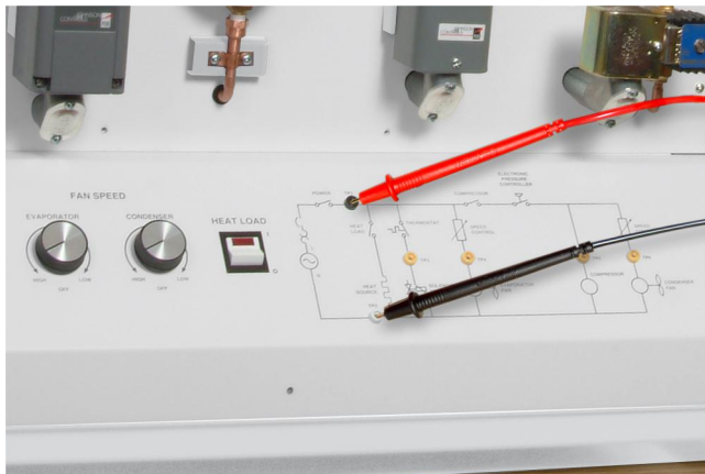
Figure 3. An electrical control panel with silk-screened diagram and banana jacks allows students to develop troubleshooting skills through the insertion of fault switches.
