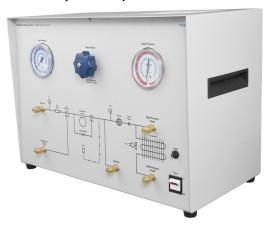
The Refrigerant Recovery Unit enables students to recover refrigerant for storage or recycling. A low-pressure indicator on the unit monitors the pressure condition on the suction side of the recovery system. A filter dryer and an oil separator are used to condition the refrigerant before it enters the recovery system compressor. At the high-pressure side of the recovery system compressor, a second oil separator ensures good lubrication by returning the oil at the
