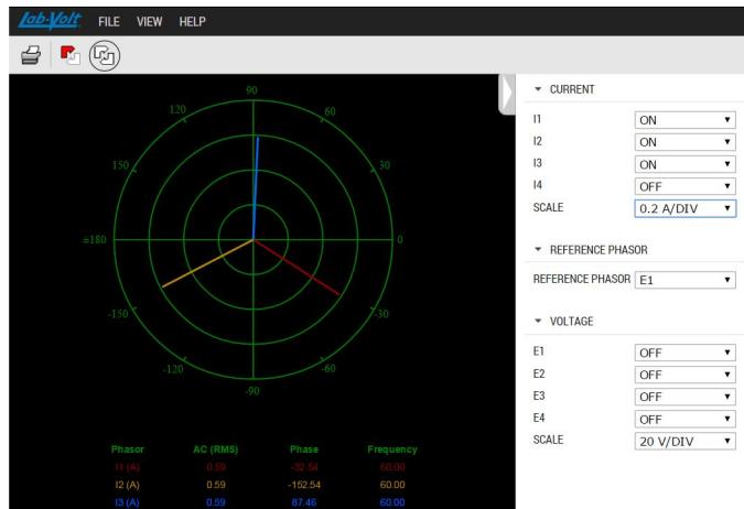
instruments. The RMS value, phase angle, and frequency of the voltage or current related to each phasor is displayed in the Phasor Analyzer window.
