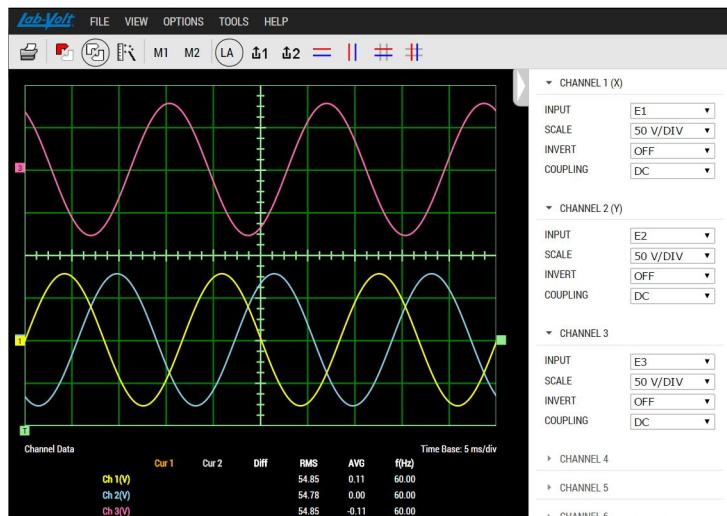
in the Oscilloscope window. Two vertical cursors can be activated to perform precise measurements at particular points on the displayed waveforms. The Oscilloscope toolbar includes two memory buttons for saving displayed waveforms.
