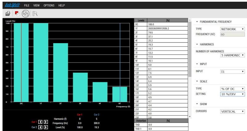
The Harmonic Analyzer allows observation and analysis of the harmonic components in the measured voltages and currents. The fundamental frequency can be manually set to the ac power network frequency or automatically set to the frequency of the fundamental component of the selected voltage or current. The harmonic components of the selected voltage or current can be displayed using a vertical scale
