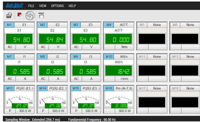
The Metering window displays up to eighteen meters, which can be configured individually for measuring ac/dc voltage and current, electrical power (active, reactive, and apparent), torque, speed, mechanical power, etc. The voltage and current meters have several modes of operation that allow measurement of the mean (dc) value, RMS value, crest factor, RMS value of a particular harmonic (up to the 15th
