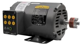
The Two-Speed Motor is a threephase, squirrel-cage, two-winding induction motor. Depending on how its two windings are connected, the motor operates at either a high-speed setting (four-pole motor) or a lowspeed setting (six-pole motor).
