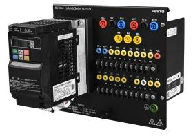
The AC Drive consists of a variable frequency speed drive with V/Hz control. The AC Drive has programmable inputs and outputs, digital and analog (for PID Control). Some electrical connections can be made using either the banana jacks or the terminal blocks.
