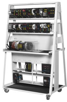
The Basic Controls Training System provides students with a complete basic training in motor controls.
