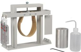
The Prony Brake is used for loading motors. The brake is complete with scales and pulley. The torque is determined from the lever arm length and the value indicated by the scales.
