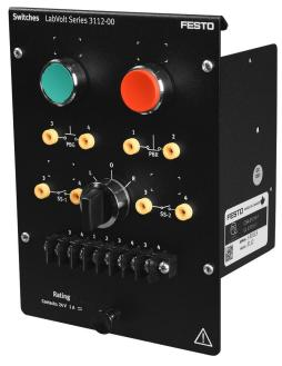
The Switches module consists of two general-purpose push buttons, one green with a normally open contact and one red with a normally closed contact, and a three-position, singlepole selector switch. Electrical connections can be made using either the banana jacks or the terminal block.
