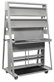
The Industrial Controls Mobile Workstation is a double-sided, mobile workstation on casters. The workstation has an A-frame configuration, is constructed of steel, and can accommodate two student groups simultaneously. Four pairs of mounting rails hold the control modules firmly in place. Additional mounting rails underneath the work surface increase the workstation storage capability. The work surface and storage shelf are protected against scratches by a rubber carpet.
