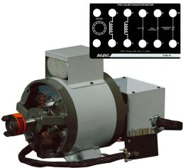
The Two-Value Capacitor Motor is fitted with a running capacitor and two running windings that are independently terminated to facilitate experimentation of various machine connections and to allow operation from a two-phase source of power. The design of this machine has been optimized so that the machine operates like a two-phase motor at full load when connected to a singlephase source.
