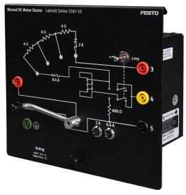
The Manual DC Motor Starter consists of a manually operated variableresistance starter. The starter can be wired as either a three- or four-point dc starter to be used with the DC Motor, Model 3179-2.
