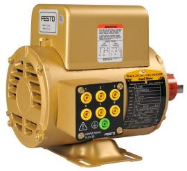
The Single-Phase Motor module consists of a single-phase, squirrelcage induction motor. A capacitor allows the motor to develop a starting torque.
