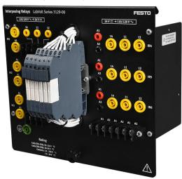
The Interposing Relays module consists of a bidirectional voltage converter for high and low control voltages. This model is equipped with three relays with 24 V dc coils and three relays with 110/120 V ac coils. Electrical connections for the lowvoltage coils and contacts can be made using either the banana jacks or the terminal blocks.
