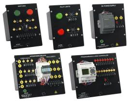
The Programmable Logic Controller Training System introduces students to the use of PLCs for motor control.
