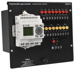
The Programmable Logic Controller consists of a small controller programmed in ladder logic with eight inputs (24 V dc) and four relay outputs. The programming is done using the LCD screen and the keypad on the controller or using the programming software (Easy-Soft) and cable included in this model. Electrical connections can be made using either the banana jacks or the terminal blocks.
