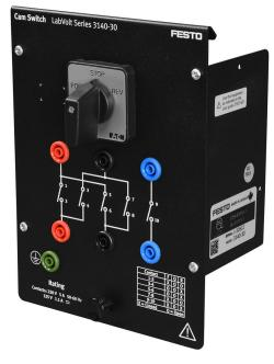
The Cam Switch consists of a manually operated drum switch. The switch control lever has three positions: Off, Forward, and Reverse. The Cam Switch is suitable for both single-phase and three-phase ac motor control. It can also be used to control series and compound dc motors.
