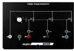
The Three-Phase Rheostat provides the mechanism for controlling motor starting torque and speed by varying the resistance in the motor circuit of the wound rotor motor. One knob adjusts the three rheostats, each of which is protected by a circuit breaker.
