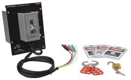
The Lockout Module consists of a lockable three-phase disconnect switch. The lockout device is a six-lock scissor type and the disconnect switch is a three-pole unit. Three padlocks and three identification tags are also included. One module is required for single-sided stations, while two are required for double-sided stations.
