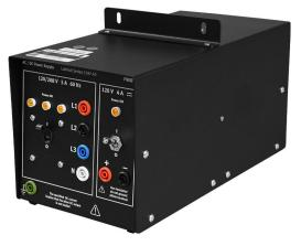
The AC/DC Power Supply provides both ac and dc power for the Industrial Controls Training System. The outlet is fed from a three-phase, four-wire breaker panel supplied elsewhere. The power supply contains input and output pilot lamps, two "on-off" switches, dual sets of four color-coded banana jacks for three-phase voltage, and dual sets of two color-coded banana jacks for fixed dc output. All outputs are circuit-breaker protected. The AC/DC Power Supply mounts on
