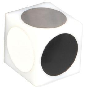
The Reflective Block consists of a block with various types of reflection surfaces: white, black, shiny metallic, matte black metallic, and retroreflective. The dimensions of the block are: 75 x 75 x 75 mm (3 x 3 x 3 in).
