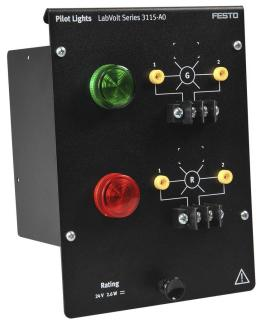
The Pilot Lights module consists of two low-power electric lights. One light is green while the other is red. Both lights are rated at a voltage of 24 V. Electrical connections can be made using either the banana jacks or the terminal block.
