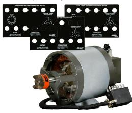
The Dahlander Two-Speed Induction Motor uses the method of pole changing based on the consequent pole principally known as the Lindström-Dahlander winding. By the insertion of the special interconnection jumper, this motor can be configured to obtain three different types of motors. Students can obtain a two-speed constant power motor, a two-speed variable torque motor, and a two-speed constant torque motor using the same motor and different
