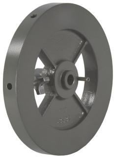
The balanced Inertia Wheel securely attaches to any 0.2 kW machine. When the inertia wheel is rotated at 1800 r/ min, it stores 790 joules of energy (550 joules at 1500 r/min).
