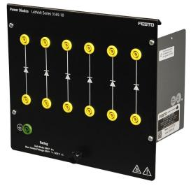
The Power Diodes module consists of six silicon rectifier diodes. The anode and cathode of all diodes are wired to independent front panel terminals, thereby allowing the diodes to be connected in any single-phase and three-phase rectifier configuration.
