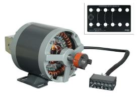
The Synchronous Motor/Generator is designed so that each phase of the stator windings of this machine is independently terminated and identified on the faceplate, allowing operation in either delta or star (wye) configuration. The rotor of this machine is equipped with a squirrelcage damper and salient pole windings in order for the machine to exhibit the same properties as
