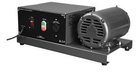
The Phase Converter converts a singlephase supply into a five-wire (wye configuration including neutral and ground) three-phase supply. This converter recreates a true three-phase power supply (with a phase voltage difference of about 10%) for threephase motor control circuits. The phase converter can supply power to
