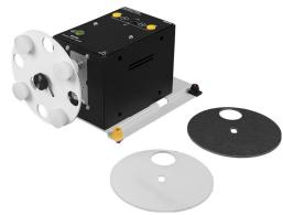
The Reversible AC Motor module consists of a reversible, single-phase gear motor having an output speed of 30 r/min. It is supplied with three perforated disks (a metallic disk, a transparent plastic disk, and a fiber disk). The disks are used to learn the characteristics of sensors. The sensors can be mounted on the motor chassis or on the work surface.
