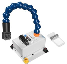
The Polarized Retroreflective Photoelectric Switch consists of a light source and a receiver combined in the same casing. This sensor requires a special retroreflective surface. The sensor is mounted on a flexible support for easy positioning. The model has one normally open and one normally closed contact, and the electrical connections are made using either the banana jacks or the terminal block.
