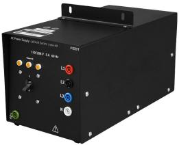
The AC Power Supply provides ac power for the Industrial Controls Training System. The outlet is fed from a three-phase, four-wire breaker panel supplied elsewhere. The power supply contains input and output pilot lamps, two "on-off" switches and dual sets of four color-coded banana jacks for three-phase voltage. All outputs are circuit-breaker protected. The AC Power Supply mounts on the upper shelf of the Mobile Workstation, Model 3103-4, and can provide power to both
