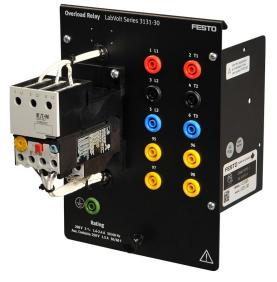
The Overload Relay consists of a threephase, bimetallic overload relay with one normally closed and one normally open contact with an adjustable setting range.
