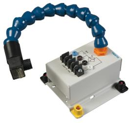
The Background Suppression Photoelectric Switch consists of a light source and a receiver combined in the same casing. The sensor is mounted on a flexible support for easy positioning. The model has one normally open and one normally closed contact, and the electrical connections are made using either the banana jacks or the terminal block.
