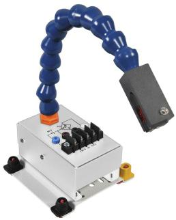
The Diffuse Reflective Photoelectric Switch consists of a light source and a receiver combined in the same casing. The sensor is mounted on a flexible support for easy positioning. The model has one normally-open and one normally-closed contact, and the electrical connections are made using either the banana jacks or the terminal block.
