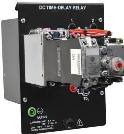
The DC Time-Delay Relay consists of a dc relay with pneumatic time-delay attachment. Delay attachment can provide on-delay or off-delay for one normally open and one normally closed contact.
