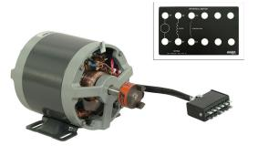
The Universal Motor has exposed commutator bars and adjustable brushes to allow students to study the effect of armature reactions and commutation while the machine is running under load. The armature winding, the series field winding, and the compensation winding are terminated independently. Students can observe the effects of both
