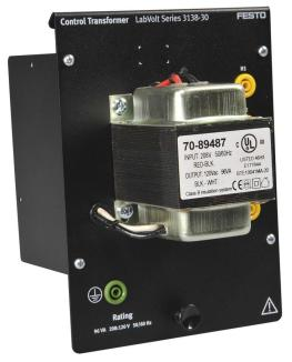
The Control Transformer converts the ac power network voltage (e.g., 208 V, 380 V, 415 V) to 110/120 V. The primary windings of the transformer are fuse-protected to prevent damage to the equipment.
