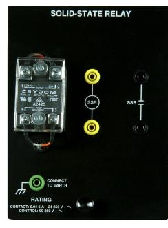
The Solid-State Relay is an industrialtype, solid-state relay designed to switch ac power loads. The switching device consists of two inverse-parallel (back-to-back) SCR's. Switching control is through an opto-isolated input and provides zero voltage switching.
