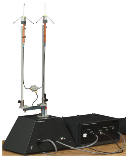
Two drooping monopole antennas installed on the ATMS Antenna Positioner ready for experimenting the effects of antenna phasing.
