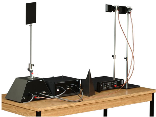
ATMS ready to measure the RCS of a metal plate. Notice the connection of a second horn antenna to the auxiliary RF input of the optional Antenna Positioner, Model 9506-A
