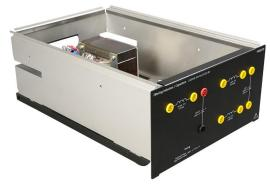
This Filtering Inductors/Capacitors module consists of two separate filters enclosed in a half-size EMS module: a low-frequency filter and a highfrequency filter. The low-frequency filter consists of an inductor and a polarized capacitor, while the highfrequency filter consists of two inductors and a non-polarized capacitor. Internal electrical components are identified on the
