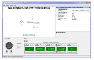
The Standard Functions (computerbased control) Set is a package of control functions that can be activated in the Four-Quadrant Dynamometer/ Power Supply, Model 8960-2, enabling the module to perform a wide variety of functions in each of its two operating modes (Dynamometer and Power Supply).
