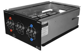
The Inductive Load consists of a module housing nine iron-core power inductors arranged in three identical banks. Each bank consists of three inductors connected in parallel that can be switched on or off with toggle switches to obtain various inductance values. This allows the equivalent inductance of each bank to be increased or decreased by steps. Six
