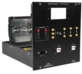
The Solar Panel Test Bench is a fullsize EMS module in which a Solar Panel, Model 8806 can be installed to perform a wide variety of tests and experiments. A powerful halogen lamp is used to illuminate the solar panel under test. The distance between the halogen lamp and solar panel can be changed to adjust the irradiance. A ventilation system is provided in the Solar Panel Test Bench to keep the solar panel at near room temperature and study the effects of temperature.
