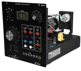
The Power Supply is enclosed in a fullsize EMS module. It can be used to power most of the EMS modules of the Electricity and New Energy Training Equipment. This Power Supply provides dc power and ac power, both fixed and variable, single-phase and three-phase. Color-coded safety banana jacks provide access to all the power sources in the Power Supply. All these power sources can be used simultaneously, provided that the total current drawn does not exceed the
