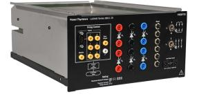
The Power Thyristors module consists of six power thyristors (SCRs) mounted in a half-size EMS enclosure. Each individual thyristor is protected against overcurrents and shortcircuits. All the anodes and cathodes of the thyristors are terminated on the front panel by color-coded, 4 mm safety banana jacks. To reduce the
