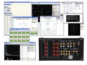
The Data Acquisition and Control Interface (DACI) is a versatile USB peripheral used for measuring, observing, analyzing, and controlling electrical and mechanical parameters in electric power systems and power electronics circuits. For these purposes, a set of computer-based instruments as well as a variety of control functions are available for the DACI. These instruments and control functions are accessed through the
