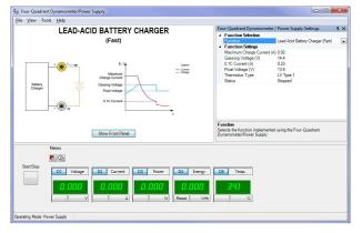
The Lead-Acid Battery Charger Function Set is a package of control functions that can be activated in the Four-Quadrant Dynamometer/Power Supply, Model 8960-2, enabling the module to implement a lead-acid battery charger, as well as a battery discharger.
