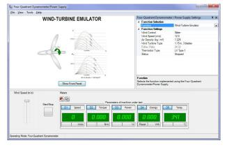
The Turbine Emulator Function Set is a package of control functions that can be activated in the Four-Quadrant Dynamometer/Power Supply, Model 8960-2, enabling the module to emulate the operation of various types of turbines.
