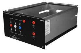
This Rectifier and Filtering Capacitors module consists of a three-phase bridge rectifier and two separate capacitors enclosed in a half-size EMS module. The bridge allows the conversion of a three-phase voltage input into an unfiltered dc voltage. This dc voltage can then be filtered using the polarized capacitors (each one protected by a diode). Internal
