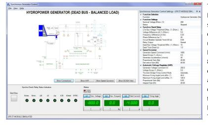
The Synchronous Generator Control Function Set enables the control of synchronous generators using different prime movers (emulated using the Four-Quadrant Dynamometer/Power Supply, Model 8960-2) and different control types for each prime mover. The function set allows the following prime movers and control types to be implemented using the Data Acquisition and Control Interface, Model 9063, and the Power Thyristors, Model 8841:
