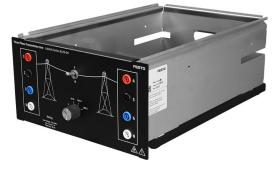
The Three-Phase Transmission Line consists of three iron-core inductors enclosed in a half-size EMS module. The inductors are specifically designed to simulate a high-voltage ac transmission line (typically 315 kV lines). The line impedance can be adjusted to four different values using a selector switch mounted on the front panel. A three-pole switch is used to
