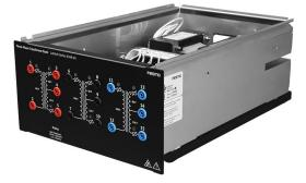
The Three-Phase Transformer Bank consists of three independent power transformers enclosed in a module. Safety banana jacks on the module front panel provide individual access to the windings of each power transformer, allowing connection in either wye or delta configuration. The transformer windings are polarized and the polarity of each winding is
