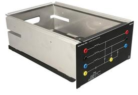
The Three-Phase Filters consists of three inductors and four capacitors enclosed in a half-size EMS module. Eight safety banana jacks on the module front panel provide access to the three-phase filter. The module is used to filter three-phase signals in power electronics applications.
