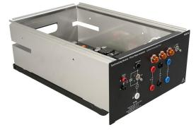
The Synchronizing Module / Three-Phase Contactor is a half-size EMS module used to control various electric devices, or synchronize two ac power sources like a synchronous generator with an ac power network. The Synchronizing Module / Three-Phase Contactor consists of a threephase contactor whose coil can be energized either manually with a toggle switch, or automatically with a
