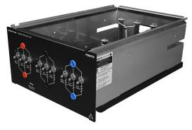
The Resistive Load consists of a module housing nine wire-wound power resistors arranged in three identical banks. Each bank consists of three resistors connected in parallel that can be switched on or off with toggle switches to obtain various resistance values. This allows the total (equivalent) resistance of each bank to be increased or decreased by steps.
