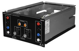
The Three-Phase Regulating Autotransformer consists of a threephase autotransformer enclosed in a half-size EMS module. Eight safety banana jacks on the module front panel provide access to both sides of the regulating autotransformer. A buck-boost selector switch can be used to increase or decrease the autotransformer output voltage by
