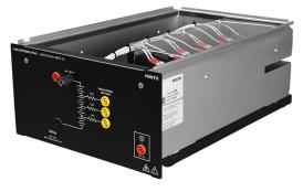
The Lead-Acid Battery Pack is a halfsize EMS module housing four 12 V lead-acid batteries connected in series. The Lead-Acid Battery Pack thus provides a fixed dc voltage of 48 V, available at two color-coded safety banana jacks on the module front panel. Three battery voltage test points allow measurement of the voltage provided by each of the four
