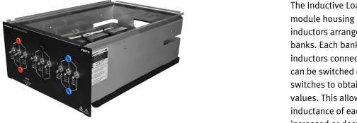
The Inductive Load consists of a module housing nine iron-core power inductors arranged in three identical banks. Each bank consists of three inductors connected in parallel that can be switched on or off with toggle switches to obtain various inductance values. This allows the equivalent inductance of each bank to be increased or decreased by steps. Six
