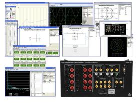
The Data Acquisition and Control Interface (DACI) is a versatile USB peripheral used for measuring, observing, analyzing, and controlling electrical and mechanical parameters in electric power systems and power electronics circuits. For these purposes, a set of computer-based instruments as well as a variety of control functions are available for the DACI. These instruments and control functions are accessed through the
