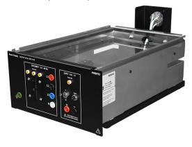
The Power Supply consists of a fixedvoltage three-phase ac power source and a fixed-voltage dc power source enclosed in a half-size EMS module. It can be used to power most of the EMS modules of the Electricity and New Energy Training Equipment. Colorcoded safety banana jacks provide access to both power sources. Independent circuit breakers, with a reset button on the front panel of the module, protect the inputs and
