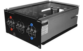
The Resistive Load consists of a module housing nine wire-wound power resistors arranged in three identical banks. Each bank consists of three resistors connected in parallel that can be switched on or off with toggle switches to obtain various resistance values. This allows the total (equivalent) resistance of each bank to be increased or decreased by steps.
