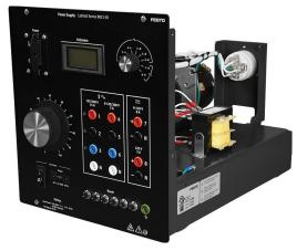
The Power Supply is enclosed in a fullsize EMS module. It can be used to power most of the EMS modules of the Electricity and New Energy Training Equipment. This Power Supply provides dc power and ac power, both fixed and variable, single-phase and three-phase. Color-coded safety banana jacks provide access to all the power sources in the Power Supply. All these power sources can be used simultaneously, provided that the total current drawn does not exceed the
