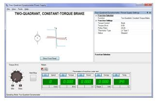
The Standard Functions (computerbased control) Set is a package of control functions that can be activated in the Four-Quadrant Dynamometer/ Power Supply, Model 8960-2, enabling the module to perform a wide variety of functions in each of its two operating modes (Dynamometer and Power Supply).
