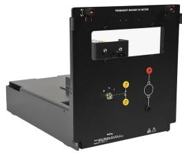
The Permanent Magnet DC Motor is a high-speed, brushed dc motor mounted in a full-size EMS module. The magnetic field required for motor operation is produced by powerful permanent magnets mounted on the motor stator. Connections to the motor are made through color-coded safety banana jacks located on the front panel on the module. Power to the motor must be fed by an external dc power source. A toggle switch mounted on the front panel can be
