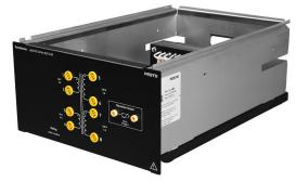
The Transformer consists of a power transformer enclosed in a module. Both the primary and secondary sides of the Transformer are made of two identical separate windings. Banana jacks on the module front panel provide access to each winding, allowing connection in a variety of configurations. The Transformer has a turns ratio of 1:5, when considering
