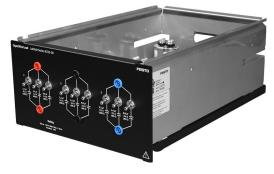
The Capacitive Load consists of a module housing nine capacitors arranged in three identical banks. Each bank consists of three capacitors connected in parallel that can be switched on or off with toggle switches to obtain various capacitance values. This allows the equivalent capacitance of each bank to be increased or decreased by steps. Six safety banana
