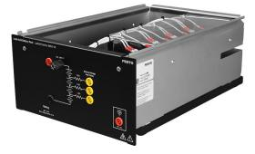
The Lead-Acid Battery Pack is a halfsize EMS module housing four 12 V lead-acid batteries connected in series. The Lead-Acid Battery Pack thus provides a fixed dc voltage of 48 V, available at two color-coded safety banana jacks on the module front panel. Three battery voltage test points allow measurement of the voltage provided by each of the four
