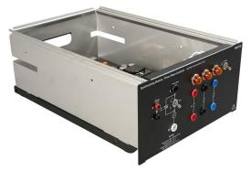
The Synchronizing Module / Three-Phase Contactor is a half-size EMS module used to control various electric devices, or synchronize two ac power sources like a synchronous generator with an ac power network. The Synchronizing Module / Three-Phase Contactor consists of a threephase contactor whose coil can be energized either manually with a toggle switch, or automatically with a
