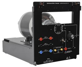
The Synchronous Motor/Generator is a 0.2 kW three-phase synchronous machine mounted in a full-size EMS module. This machine can be operated either as a three-phase motor or a three-phase generator. Each phase of the machine stator windings is independently terminated and identified on the front panel to allow operation in either wye or delta configuration. The machine rotor is equipped with a squirrel-cage damper. Variable dc excitation to the rotor field
