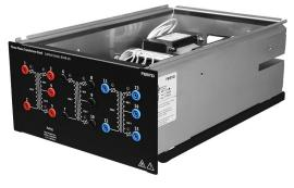
The Three-Phase Transformer Bank consists of three independent power transformers enclosed in a module. Safety banana jacks on the module front panel provide individual access to the windings of each power transformer, allowing connection in either wye or delta configuration. The transformer windings are polarized and the polarity of each winding is
