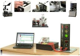
PLC Applications, Series 8075, aim to further develop the students' understanding of PLC programming. These small-scale systems are typical of what can be found in the industry. The systems' training capabilities are enhanced by their modularity and their instructor-inserted faults.
