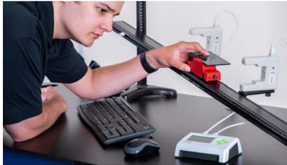
The datalogger included is fully self-contained and has a VGA output for connection to a projector for class demonstrations.
