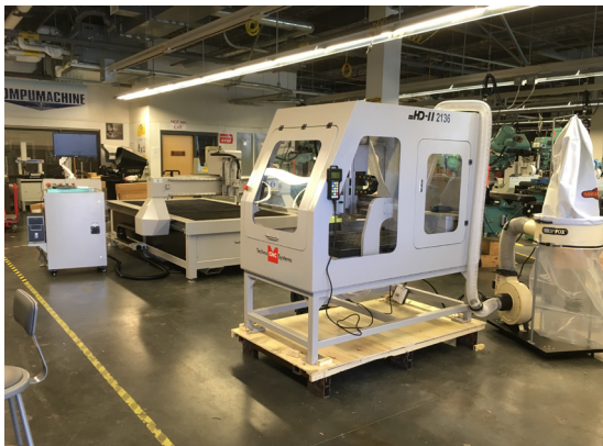
Safety Enclosure: Techno's heavy duty steel base includes hand jack center cross strut for easy maneuverability. Techno's safety enclosure feature ergonomic front main door with vertical swing, two side doors, (8) enclosure viewing windows, and 3.0" top dust collection port. Techno's HD-II Table top router with stand and enclosure is designed to roll through a standard 36" door opening.
