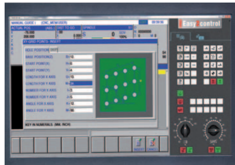
The change to a different control system is carried out within a minute by calling up the respective software
