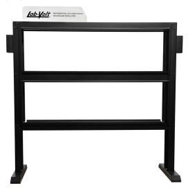
The workstation allows two student groups to work simultaneously. The structure is pre-assembled, made of steel, and intended for use on a table (not supplied, offered as option). Four pairs of mounting rails firmly hold the modules of the HVAC-R line of products in place. One holder on each side permits users to neatly arrange the test leads. A touch-screen computer mount (not supplied, offered as option) can be attached to either side.
