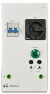
The Power Source provides power to the other modules of the training system through two 4 mm terminals. The module can be powered via standard single-phase ac power outlets. The power source output voltage is equal to the voltage of the ac power network to which the power source is connected. A thermal-magnetic circuit breaker provides overcurrent and short-circuit protection.
