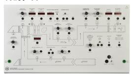
The Building Energy Management Training System is the main module of the training system. It represents the infrastructure of a building to which the programmable controllers connect. The faceplate of this module represents the building rooftop unit, the various temperature and pressure sensors, and the infrastructure of the building (including the zone damper, hot water reheater, zone sensors, lighting system, and baseboard heater).
