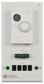
The Temperature Network Sensor introduces students to the notion of remote temperature set points and familiarizes them with SA bus networks. In a large building, sensors of this type are typically networked to provide temperature information to the controllers. The module also includes four fault-insertion switches to teach the principles of troubleshooting, as well as two ground terminals.
