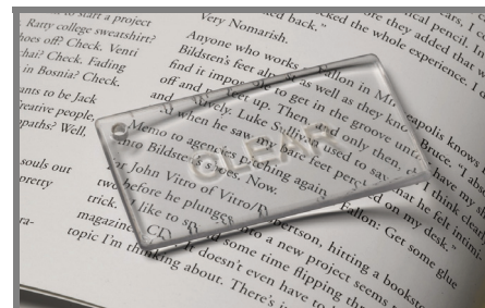
Image 1: Sample of polished and lacquered Objet VeroClear
