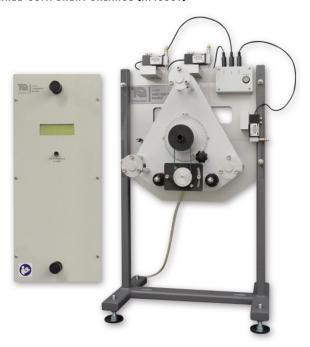
The Three-Component Balance fits onto the working section of TecQuipment's Subsonic Wind Tunnel (AF1600).
