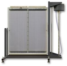
A 36-tube tilting manometer for measuring pressure in subsonic wind tunnels, including TecQuipment's AF1600. A backboard with a graduated scale holds each manometer tube.
