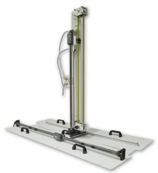
This is an X/Y traverse Pitot-static unit that fits to the top of the working section of the AF1600. It connects to VDAS® for the display of the Pitot-tube pisition (in both axes). The pressure tapping may be connected to AFA6, the 32-Way Pressure Display Unit (included) for electronic display and to link with VDAS®.
