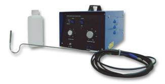
The smoke generator and probe is an optional ancillary to allow the observation of airflow in subsonic wind tunnels and other airflow situations.
