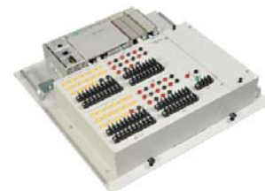
AB CompactLogix PLC
